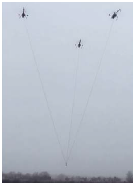
Figure 3: Load Transportation Using Three UAVs (mbernard79, 2007).
